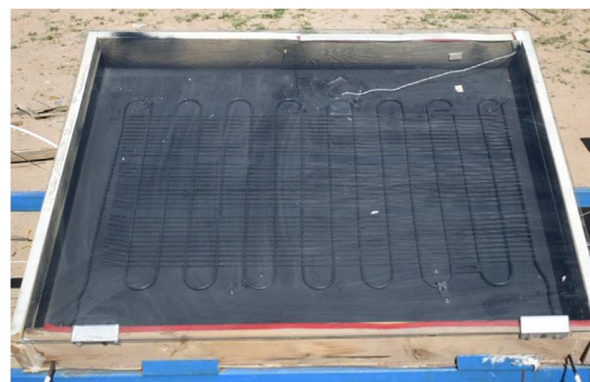
Fig. 2. Pictorial view finned tube solar collector.
