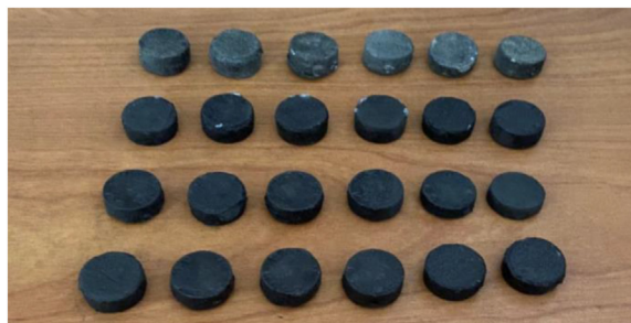
Fig. 3. Shape of samples used for the \gamma -ray attenuation measurements.
