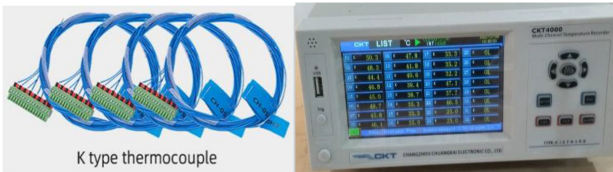
Fig. A4. Data logger and k-type thermocouple.
